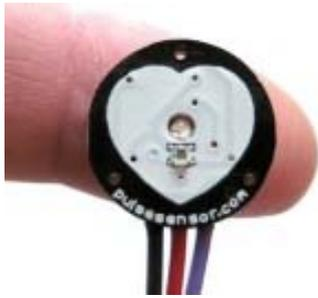
Fig. 3. Pulse sensor.
