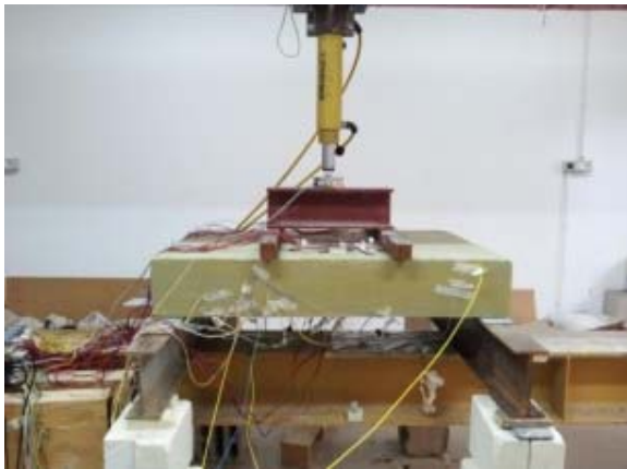
Fig. 8. Out-of-plane flexural test set-up on masonry walls.
