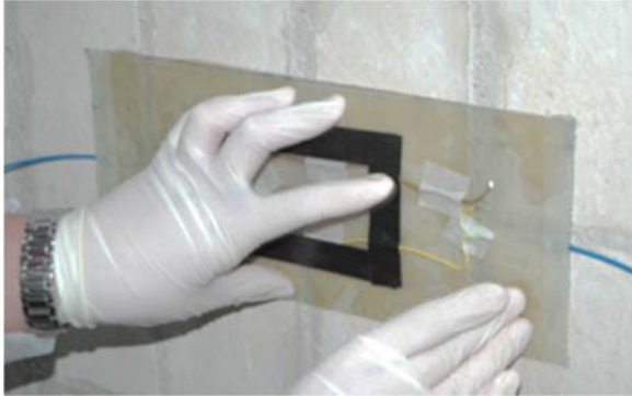
Fig. 1. Smart Patch application on masonry wall.
