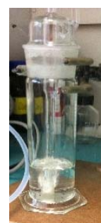
Fig. 5. The ionic liquids based filter and bubbling process.
