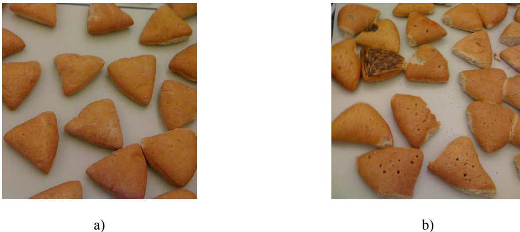
Fig. 4. Sample of products without known inspection presets: a) acceptable products, b) unacceptable products.
