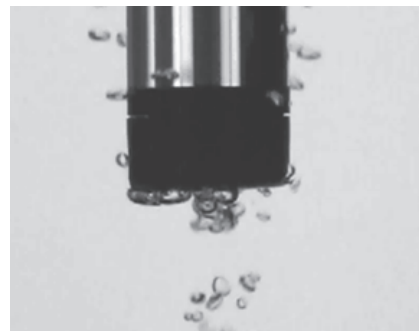
Fig. 10. Effect of bubbles on the measurement results.
