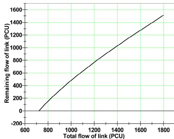
Fig. 2. Image of function between remaining flow of link and total flow of link (the range from 720 to 1800).
