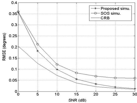
Fig. 3. RMSEs of  $\hat{\phi}_i$  estimated by the proposed and SOS methods versus SNR.
