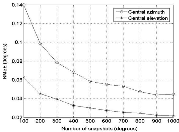
Fig. 4. RMSEs of  $\hat{\theta}_i$  and  $\hat{\phi}_i$  estimated by the proposed method versus snapshots.
