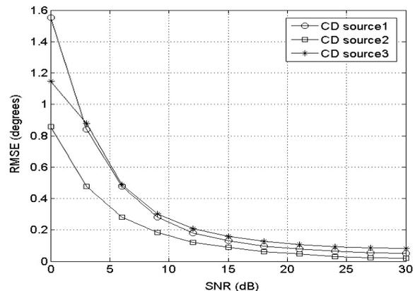
Fig. 7. RMSEs of  $(\hat{\theta}_i, \hat{\phi}_i)$  estimated by the proposed method versus SNR for three CD sources.
