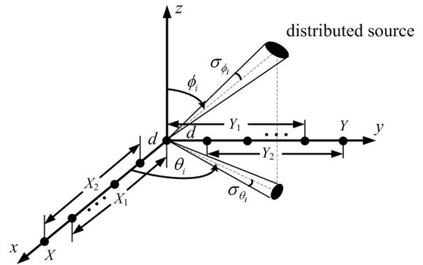
Fig. 1. L-shape array geometry.
