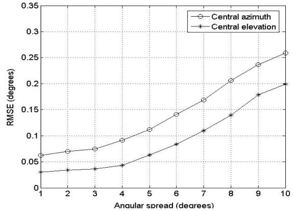
Fig. 5. RMSEs of  $\hat{\theta}_i$  and  $\hat{\phi}_i$  estimated by the proposed method versus angular spread.
