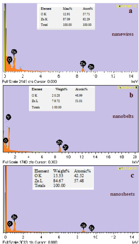
**Fig. 3.** EDX images of different morphologies of ZnO Nanostructures: (a) Undoped ZnO Nanowires; (b) Cu doped ZnO Nanobelts; (c) Cu doped ZnO Nanosheets.
