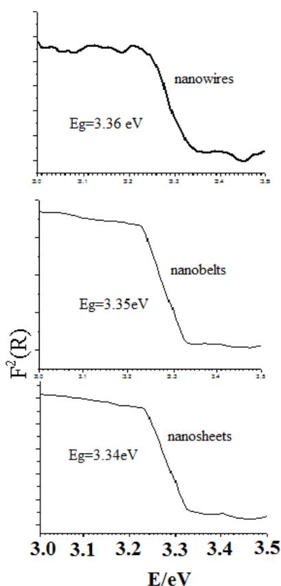
**Fig. 5.** Absorption spectroscopy results after Kubelka-Munk treatment of (a) Undoped ZnO Nanowires; (b) Cu doped ZnO Nanobelts; (c) Cu doped ZnO Nanosheets.
