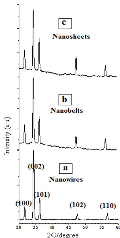
**Fig. 4.** XRD result of different morphologies of ZnO Nanostructures: (a) Undoped ZnO Nanowires; (b) Cu doped ZnO Nanobelts; (c) Cu doped ZnO Nanosheets.
