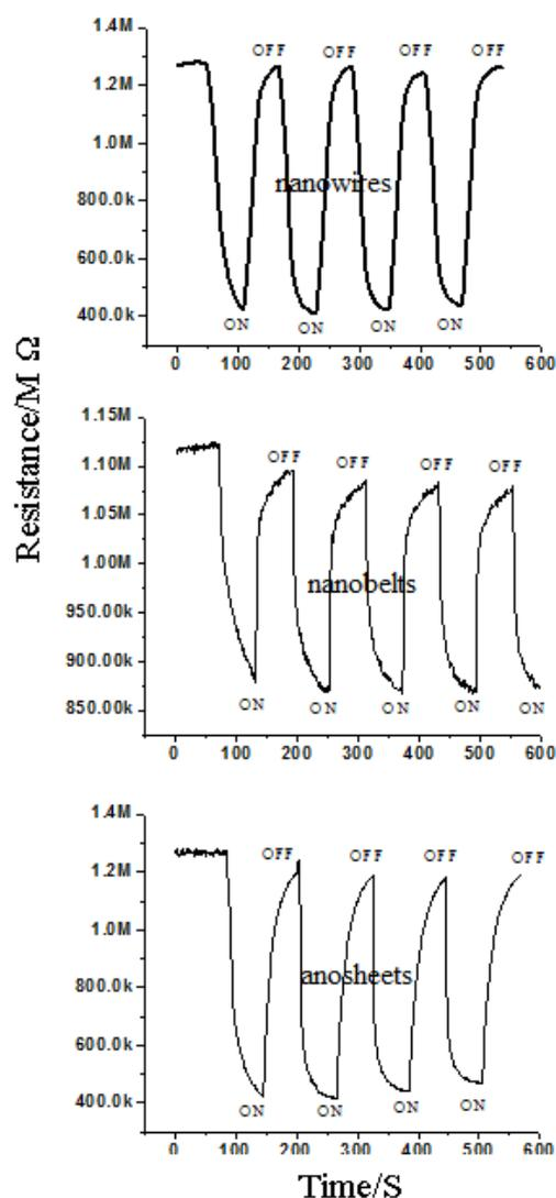
**Fig. 1.** UV sensing results of different morphologies of ZnO Nanostructures: (a) Undoped ZnO Nanowires; (b) Cu doped ZnO Nanobelts; (c) Cu doped ZnO Nanosheets.
