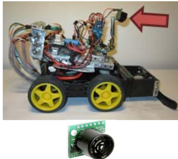
**Fig. 10.** The lawn mower device with the Ultrasonic sensor placed at the top right side.
