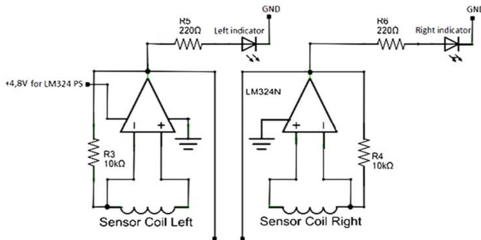
Fig. 16. On board coil sensors circuitry.
