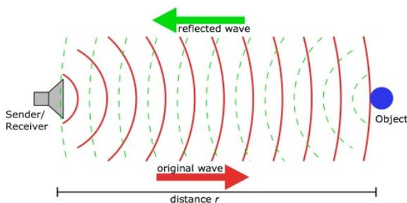
Fig. 4. The Ultrasonic sensor function.
