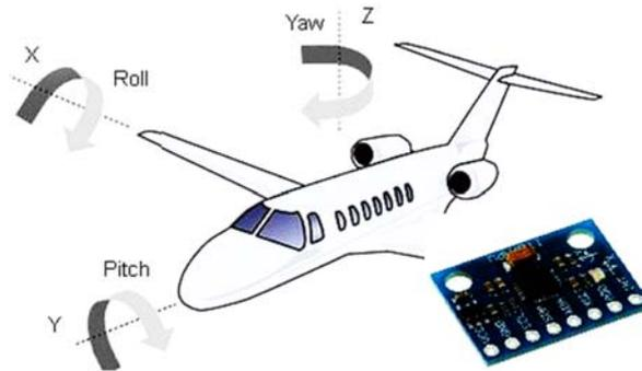
**Fig. 7.** A common Gyroscope to measure 3 axis rotation.
