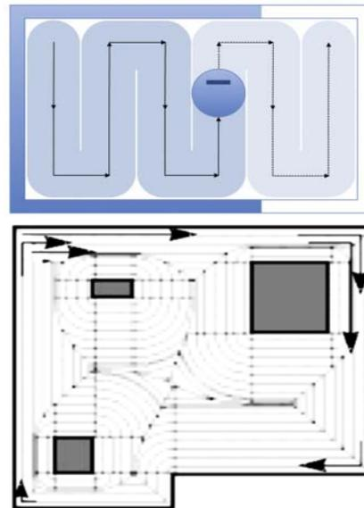
Fig. 13. Zig-Zag and Contour shrinking path method.
