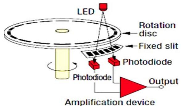
**Fig. 9.** Optical Encoders principles.
