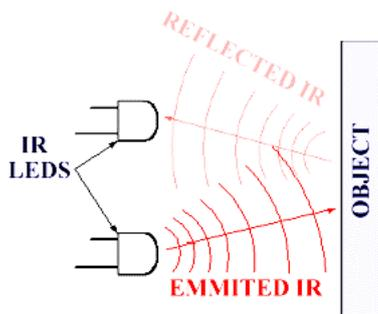
Fig. 3. The IR sensor operation schematic.
