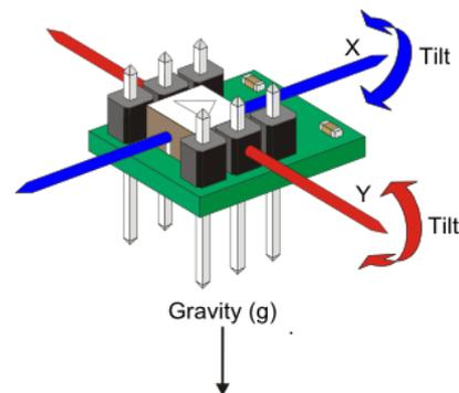
Fig. 6. A typical Accelerometer layout.
