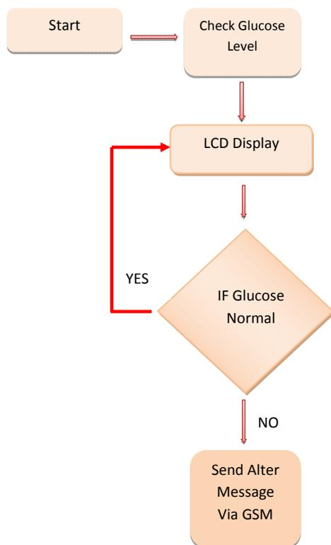
Fig. 4. Flow Diagram of Hardware Implementation.
