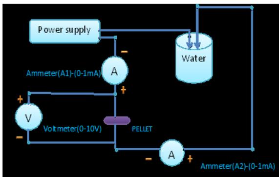
Fig. 2. Circuit Diagram for conductivity measurement.
