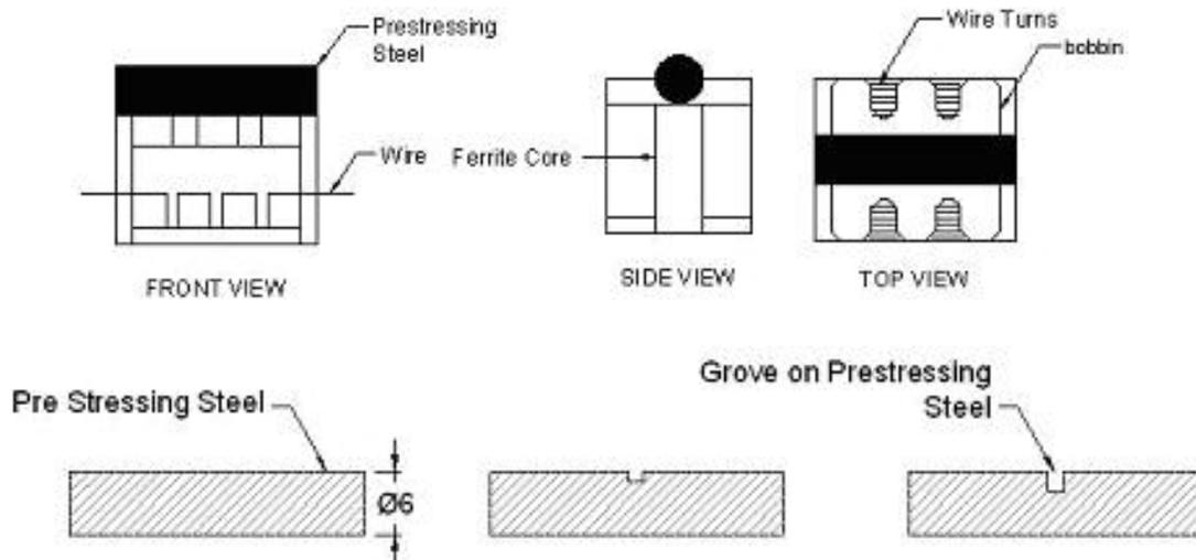
Fig.1. Schematic of eddy current sensor.
