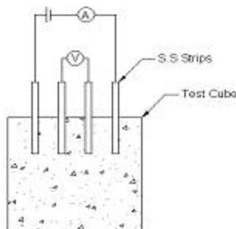
Fig.3.Schematic of resistivity sensor.
