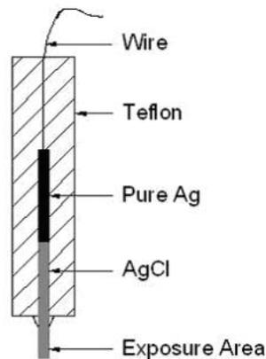
Fig.2.Sketch of embeddable chloride sensor.
