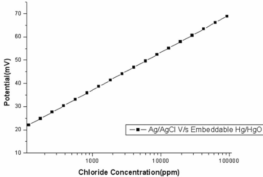
Fig.6.Chloride profile for the Ag/AgCl sensor.
