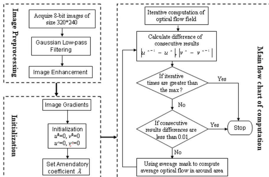
Fig. 1. The flow chart of calculation of optical flow.
