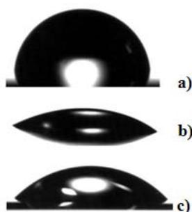
**Fig. 3.** Surface wettability for: a) bare gold, b) MHDA treated gold microelectrode, and c) immobilization of mAb-TNF- $\alpha$  onto the gold microelectrode.
