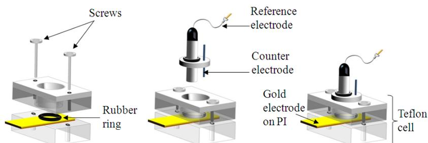
**Fig. 2.** Scheme (from left to right) showing all Teflon cell elements, which will be connected to the VMP3 for electrochemical measurement (CV and EIS).
