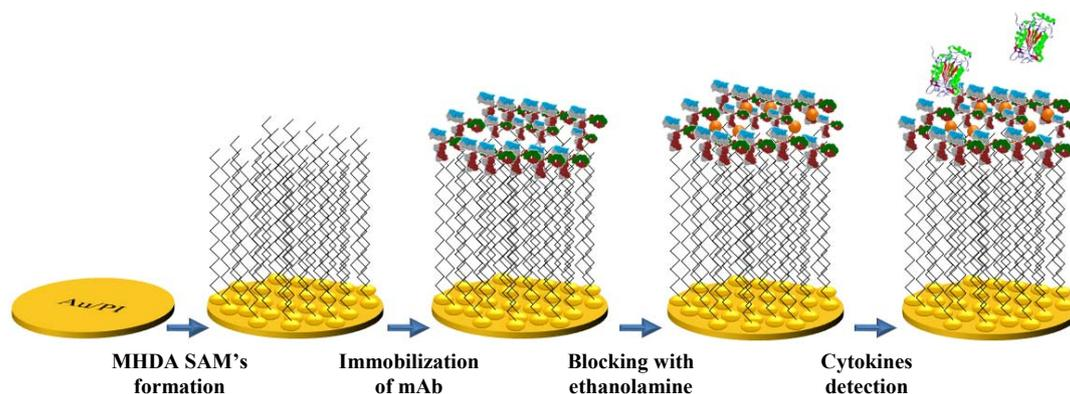
**Fig. 1.** Schematic representation of the mAb-TNF- $\alpha$  immobilization on a gold electrode modified with MHDA starting by: The formation of MHDA SAMs on a gold substrate; the activation of carboxylic acid functional groups with a solution of EDC/NHS; coupling the mAb-TNF- $\alpha$  to the activated SAMs through amino-acid bonding; blocking the residual activated groups with ethanolamine; and detection of the corresponding cytokine.
