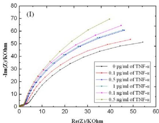
**Fig. 5.** Nyquist plot impedance ( $Z_r$  vs.  $Z_i$ ) vs. SCE at 5 mM of  $K_3[Fe(CN)_6]/K_4[Fe(CN)_6]$  in PBS (pH 7.4) at various human TNF- $\alpha$  concentrations detected by the corresponding mAb: (●) 0 pg/mL; (◐) 0.1 pg/mL; (▲) 0.5 pg/mL; (▼) 1 pg/mL; (◄) 0.1 ng/mL; and (►) 0.5 ng/mL.
