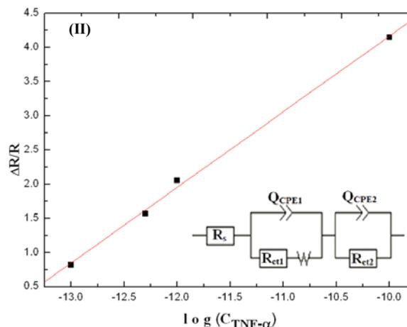
**Fig. 6.** The normalized transfer resistance of transfer charge vs. the log of human TNF- $\alpha$  concentrations. The parameter  $\Delta R/R$  was given as  $(R_{ct2-Ag} - R_{ct2-Ab})/R_{ct2-Ab}$ , where  $R_{ct2-Ab}$  represents the charge transfer resistance when Anti-TNF- $\alpha$  is immobilized on the SAM/Au electrode, and  $R_{ct2-Ag}$  corresponds to the charge transfer resistance at different TNF- $\alpha$  Ag concentrations.
