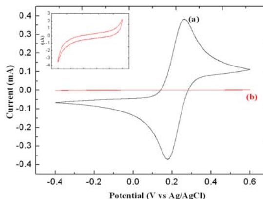
**Fig. 4.** CV for bare gold and mixed SAM electrodes in 5 mM  $\text{K}_3[\text{Fe}(\text{CN})_6]/\text{K}_4[\text{Fe}(\text{CN})_6]$  in PBS (pH 7.4). Electrodes were scanned at a rate of 100 mV/s with (a) bare gold electrode and (b) mixed SAMs of MHDA covered electrode. This confirms the functionalization of the gold microelectrodes. (Inset shows the magnification of the curve (b)).
