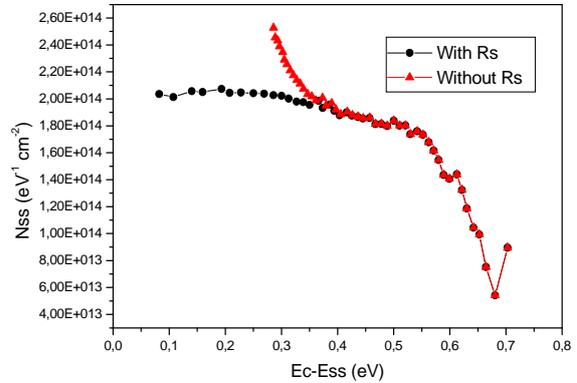
Fig. 3. The energy density distribution profile of the Au/Ni-AlInN Schottky diode.
