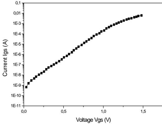
Fig. 2. Gate leakage current  $I_{gs}(V_{gs})$  of the HEMT.
