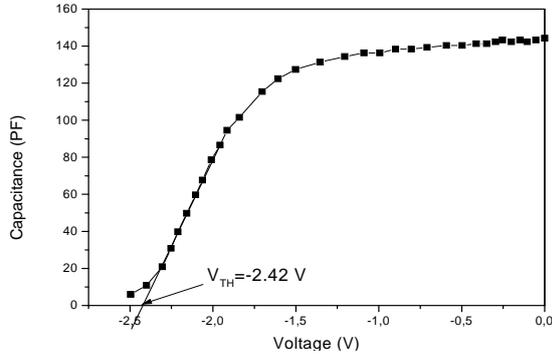
Fig. 4. The capacitance of the AlInN/GaN HEMT.
