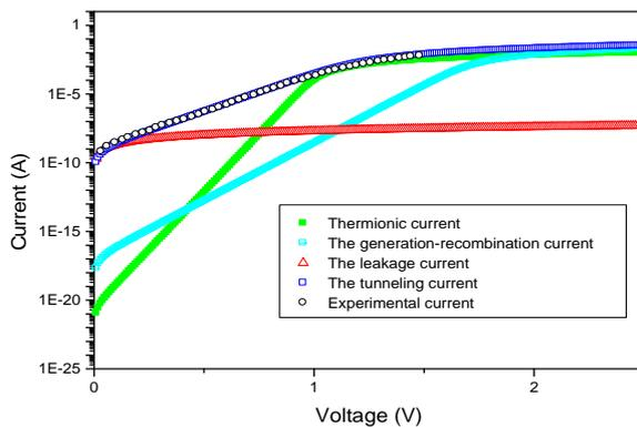
**Fig. 7.** Characteristics  $I(V)$  following experimental and theoretical contribution of each current of the Ni/Au/AlInN/GaN structure.
