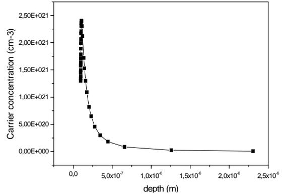
Fig. 5. The carrier concentration profile versus the depth  $W$  of the AlInN/GaN HEMT.
