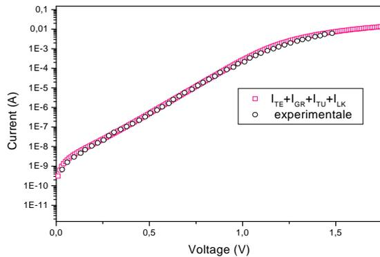
**Fig. 6.** Characteristics  $I(V)$  experimental and theoretical of the Ni/Au/AlInN/GaN structure.
