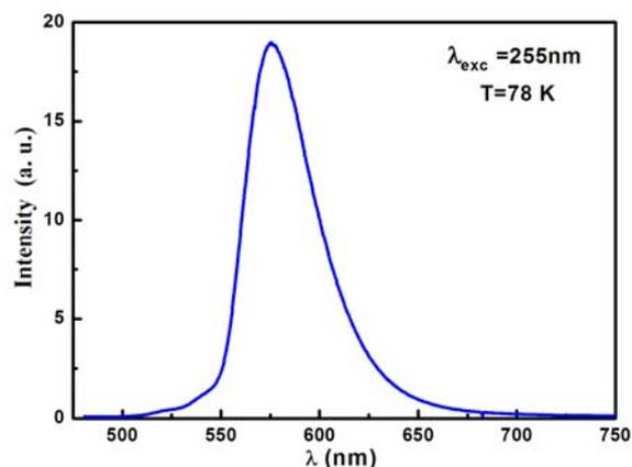
**Fig. 4.** PL spectrum of a typical  $\text{SiO}_2/\beta\text{-Zn}_2\text{SiO}_4$ :Mn nanocomposite.
