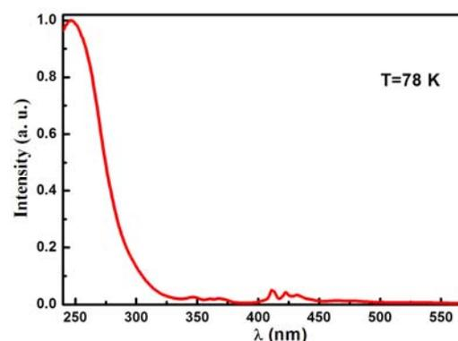
**Fig. 5.** PLE spectrum of a typical  $\text{SiO}_2/\beta\text{-Zn}_2\text{SiO}_4$ :Mn nanocomposite.
