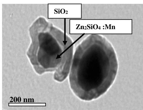
**Fig. 3.** TEM photograph showing the general morphology of the  $\text{SiO}_2/\beta\text{-Zn}_2\text{SiO}_4$ :Mn nanocomposite.
