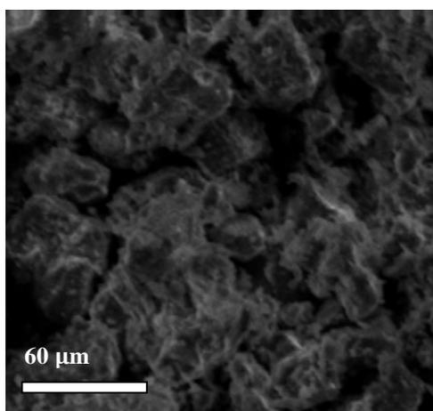
**Fig. 2.** SEM photograph showing the general morphology of the  $\text{SiO}_2/\beta\text{-Zn}_2\text{SiO}_4$ :Mn nanocomposite.
