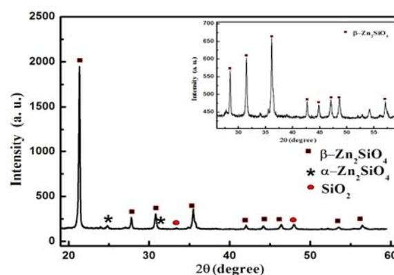
Fig. 1. X-ray diffraction pattern of the SiO<sub>2</sub>/β-Zn<sub>2</sub>SiO<sub>4</sub>:Mn nanocomposite.
