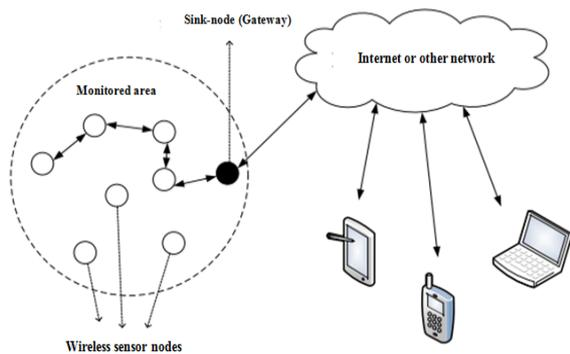
Fig. 1. Structure of wireless sensor network.
