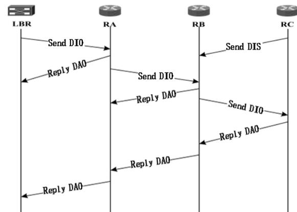
Fig. 2. Simplified building process of DODAG.
