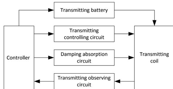
Fig. 1. Structure of the transmitter.
