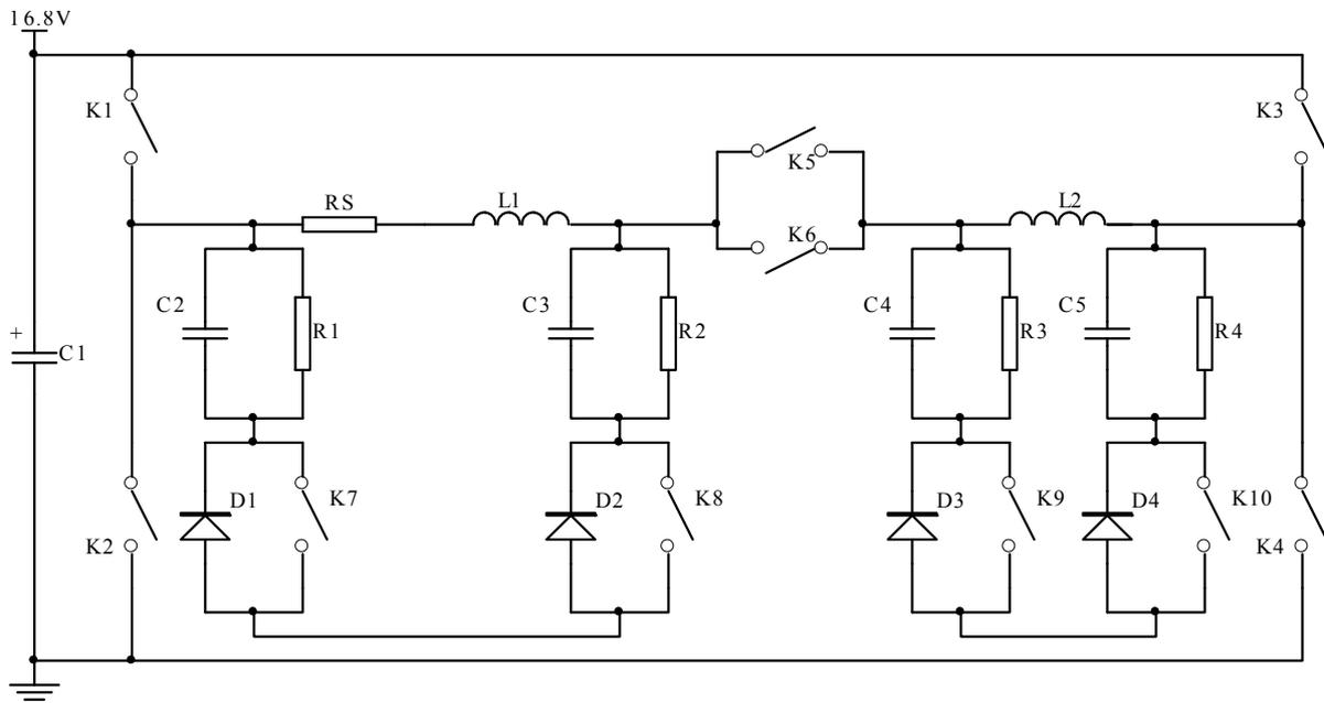
Fig. 2. Structure of transmitting coil circuit.
