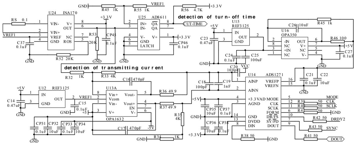
Fig. 4. Acquisition circuit of transmitting current.
