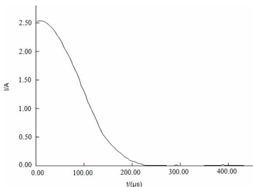
Fig. 5. Waveform of transmitter current falling edge.
