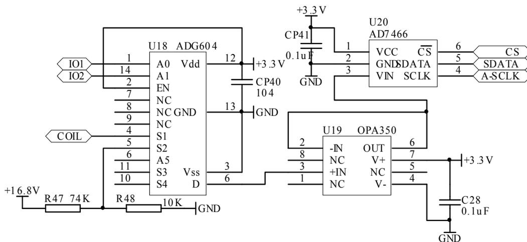
Fig. 3. Detection circuit of transmitting coil and voltage.
