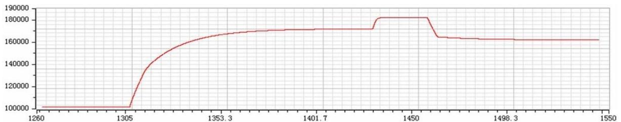
Fig. 10. Pressure closed-loop control response curve.
