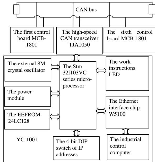
Fig. 4. Hardware block diagram of control host YC-1001.
