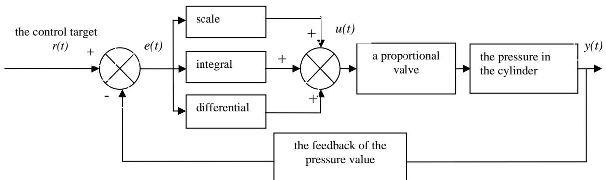
Fig. 2. PID control block diagram.
