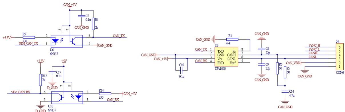
Fig. 6. CAN bus interface circuit.
