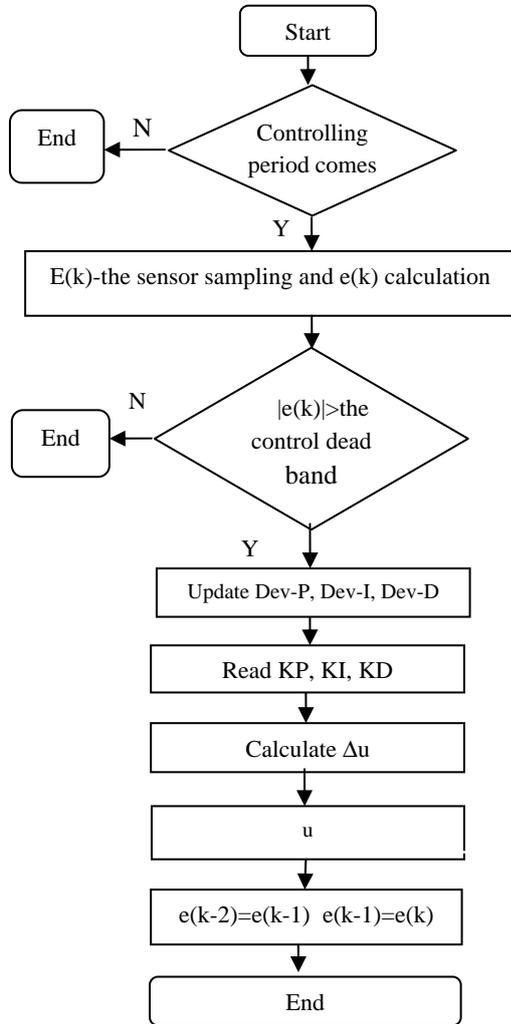
Fig. 3. The flow of incremental PID algorithm with dead zone control.
