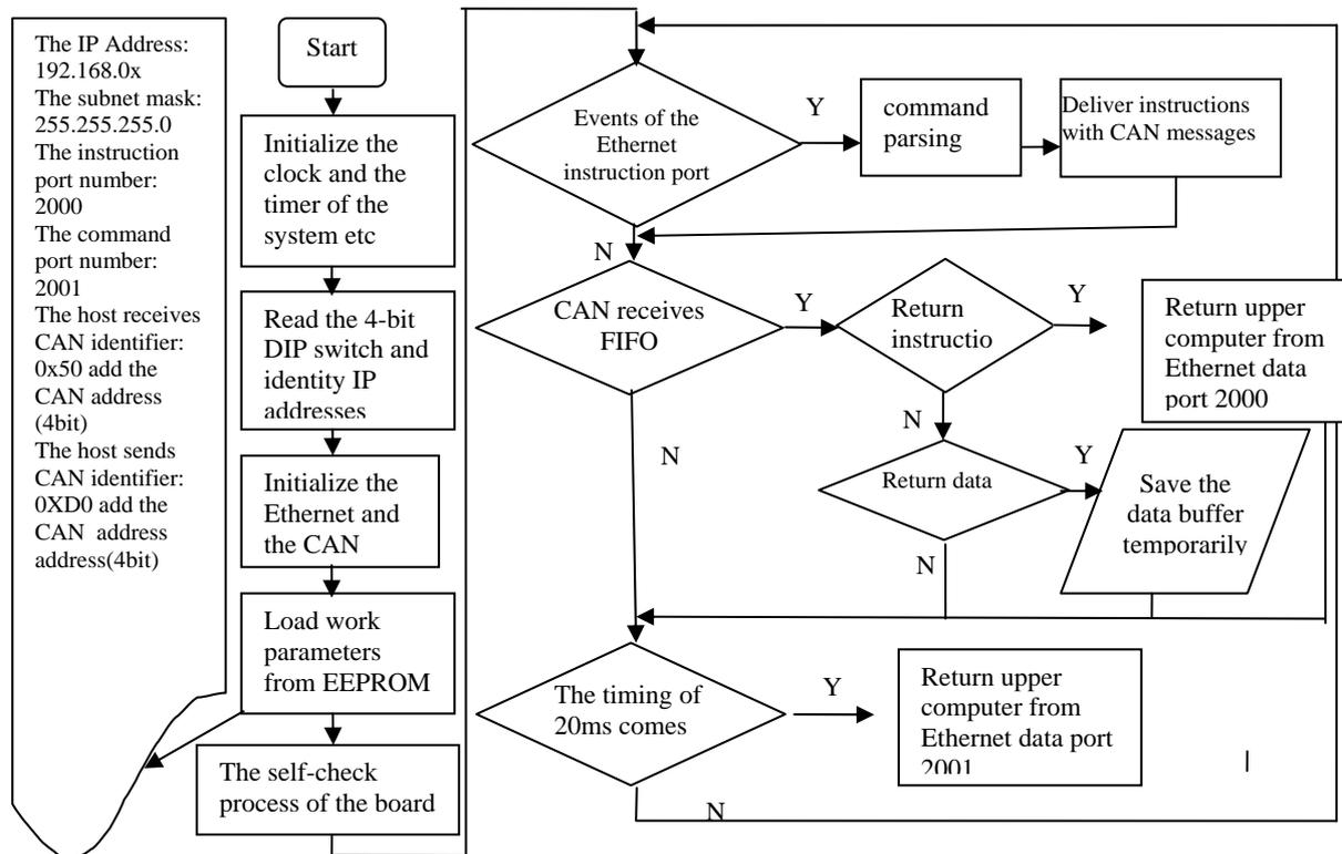
Fig. 7. Main program flow of control mainboard.
