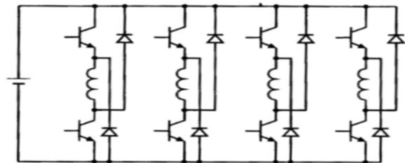
Fig. 4. The inverter circuit design of switch reluctance drive electromotor.
