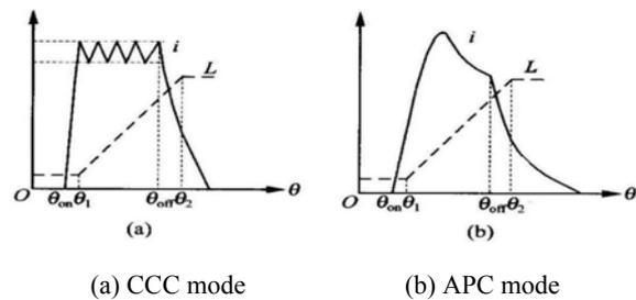
Fig. 3. The current and voltage waveform in the CCC and APC mode.
