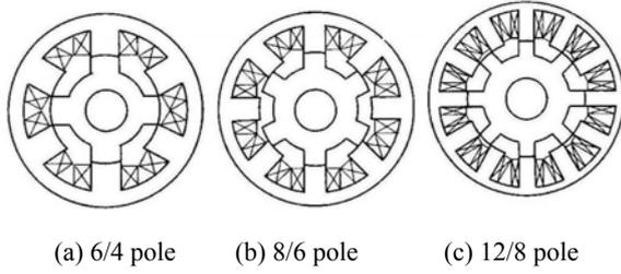
Fig. 1. The basic structure of switch reluctance electromotor.
