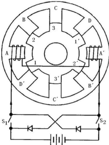
Fig. 2. Four-phase 8/6 pole switch reluctance drive electromotor.
