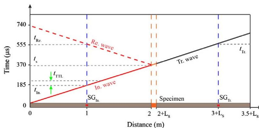
Fig. 2. Lagrangian wave propagation diagram.
