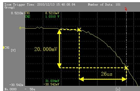
Fig. 4. The pre trigger time measurement.
