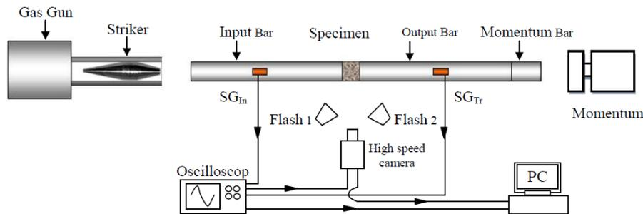
Fig. 1. Schematic of the split Hopkinson pressure bar system.
