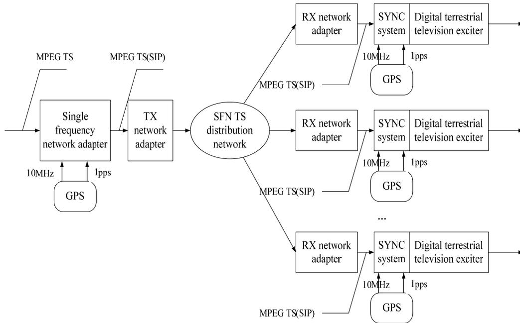
Fig. 1. Sketch map of digital terrestrial television broadcasting single frequency network architecture.
