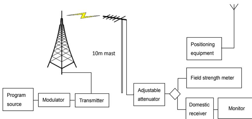
**Fig. 6.** Sketch map of simplified measurement system.
