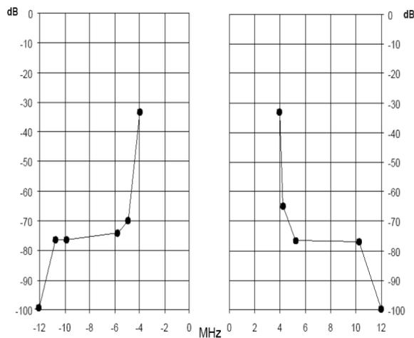
Fig. 3. Spectrum masks for a digital terrestrial television transmitter operating on an upper or down adjacent channel to a co-sited analog television transmitter.
