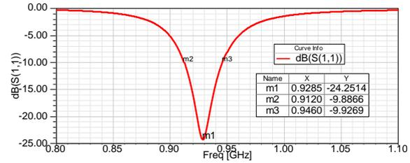
**Fig. 4.** Return Loss versus frequency characteristic of initial antenna.
