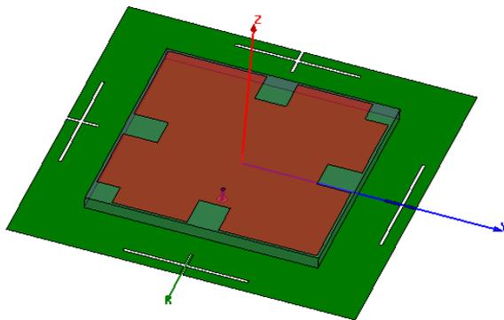
**Fig. 3.** Simulation model for the designed antenna in HFSS.
