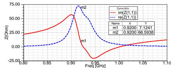
**Fig. 5.** Input impedance versus frequency characteristic of initial antenna.
