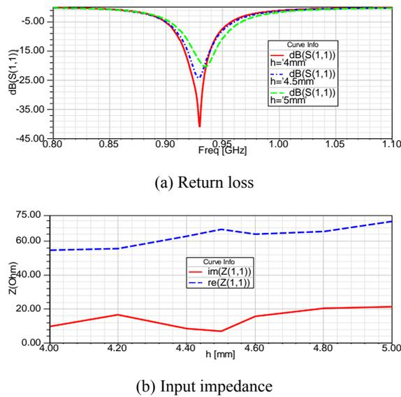
**Fig. 10.** Effect of substrate thickness H on antenna performances.
