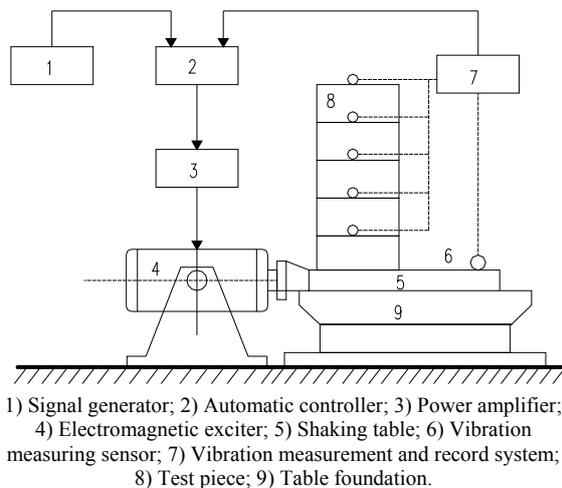
Fig. 2. Composition system of the shaking table.
