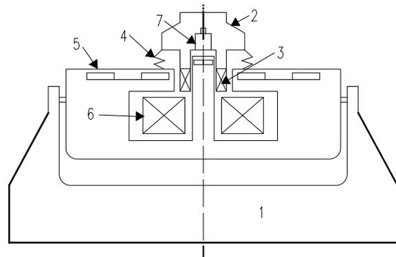
1) Frame; 2) Vibration exciter head; 3) Driving coil; 4) Supporting spring; 5) Magnetic shield; 6) Exciting coil; 7) Sensor
