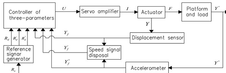
Fig. 5. Schematic diagram of the shaking table servo system with the controller of three parameters
