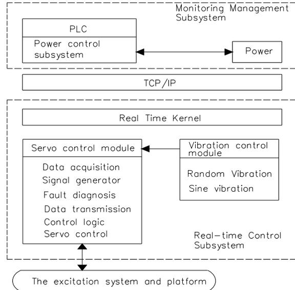
Fig. 4. System software structure.
