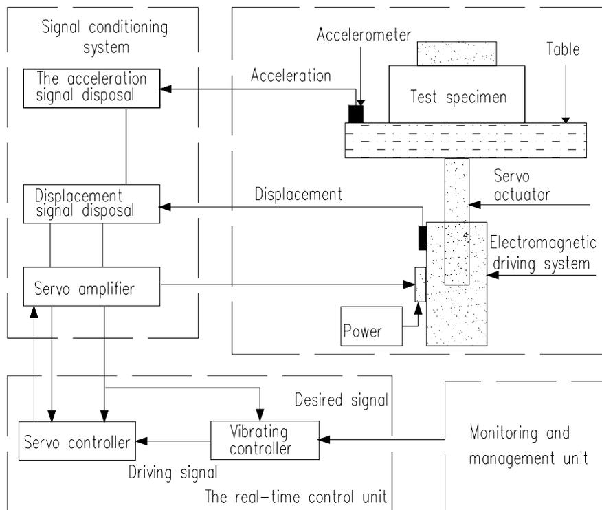
**Fig. 1.** Components of shaking table seismic test system.
