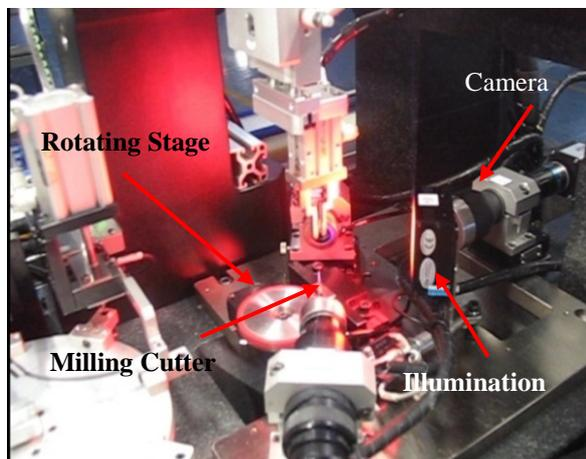
Fig. 2. Physical figure of milling cutter visual inspection system.
