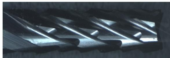
**Fig. 1.** Physical figure of micro-milling cutter.
