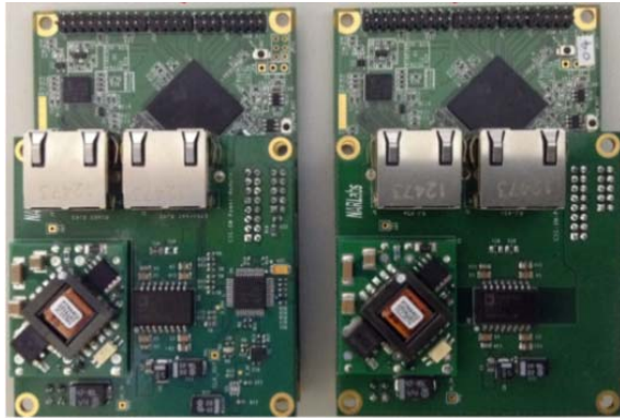
Fig. 4. The pictures of printed circuit boards of gateway (left) and sensor node (right).
