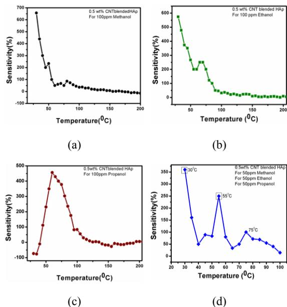
**Fig. 9.** Sensor sensitivity at different temperature of 0.5 wt% CNT blended HAp sensor substrate (a) in the presence 100 ppm methanol (b) in the presence 100 ppm ethanol (c) in the presence 100 ppm propanol and (d) in presence of mixture of organic vapors (methanol, ethanol, and propanol) to obtain the operating temperature.
