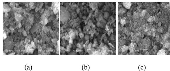
**Fig. 1.** SEM micrographs for native HAp and CNT blended HAp (a) Native HAp, (b) 0.5 wt% CNT blended HAp, (c) 0.7 wt% CNT blended HAp.
