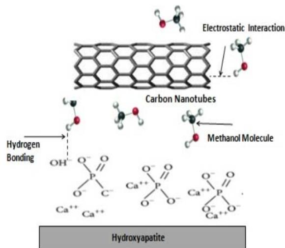
Fig. 4(b). Formation of hydrogen bonding, due to dipole-dipole interaction between polar methanol molecule and hydroxyl ions on HAp surface. Electrostatic interaction between methanol and CNT molecules leads to enhancement in the sensing property of the substrate material.
