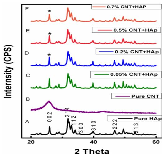
Fig. 2. X-ray diffraction pattern of native HAp, CNT and CNT blended HAp material (\* represents the peak for CNT): Y-axis has arbitrary units.
