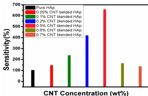
Fig. 5. Variation in sensitivity of methanol vapours for different CNT concentrations in HAp, at room temperature (30°C) for 100 ppm methanol.
