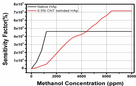
**Fig. 7.** The sensitivity of native HAp and 0.5 % CNT blended HAp thick films for various concentrations of methanol vapours at room temperature (30°C).
