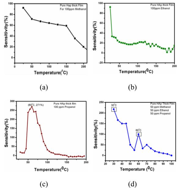
**Fig. 8.** Sensor sensitivity at different temperature of native HAp sensor substrate (a) in the presence 100 ppm methanol (b) in the presence 100 ppm ethanol (c) in the presence 100 ppm propanol and (d) in the presence of a mixture of organic vapors (methanol, ethanol, and propanol) to obtain the operating temperature.
