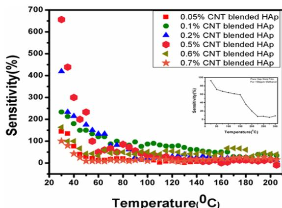
Fig. 4(a). Sensor sensitivity (response) of native HAp and CNT blended HAp at variable temperature for 100 ppm concentration of methanol.
