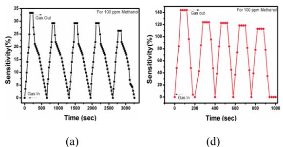
Fig. 6. Response / recovery time plot for native HAp and 0.5 wt% CNT blended HAp thick films in the presence of 100 ppm methanol; Continuous repeated cycles for response / recovery time at room temperature (30°C), (a) native HAp, (b) 0.5 % CNT blended HAp.
