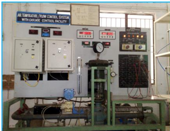
Fig. 8 (a). Laboratory Air Flow Control System.
