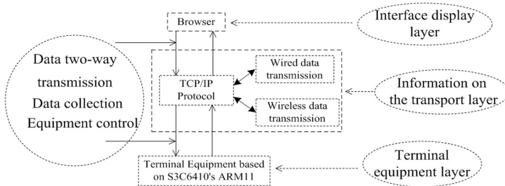
Fig. 1. Structure diagram of the whole system.
