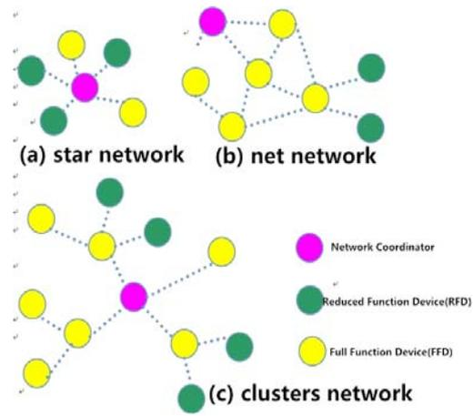
Fig. 3. Three main types of wireless network.
