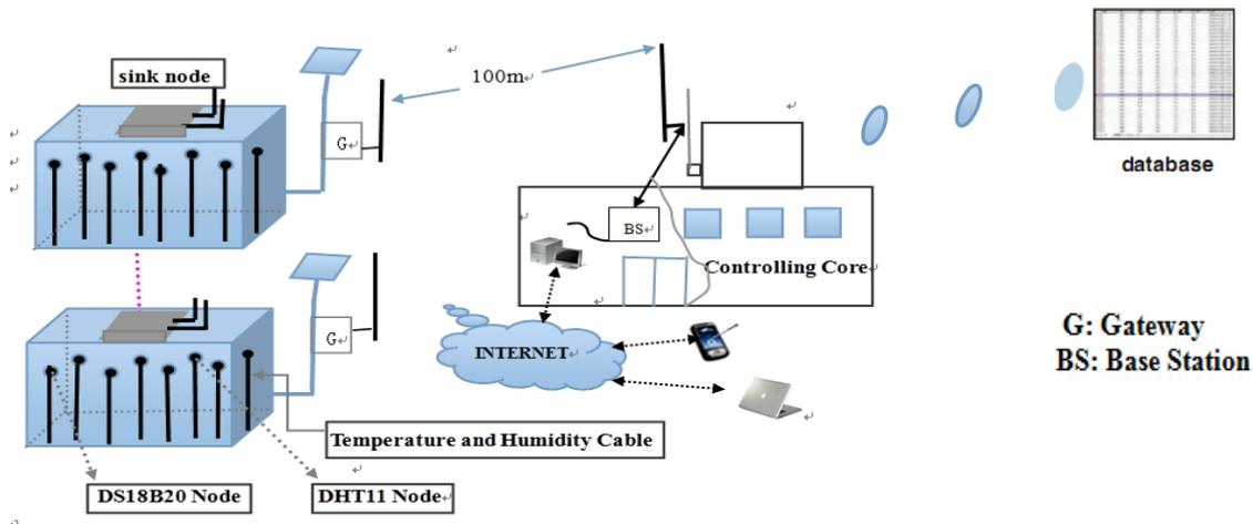
Fig. 4. Architecture proposed for the monitoring of granary.
