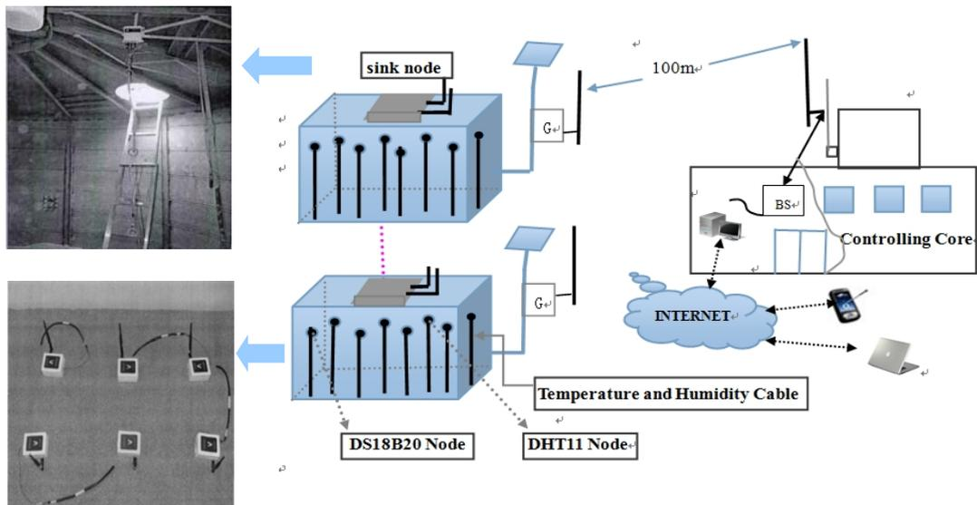
Fig. 7. The overall layout of actual testing granary.
