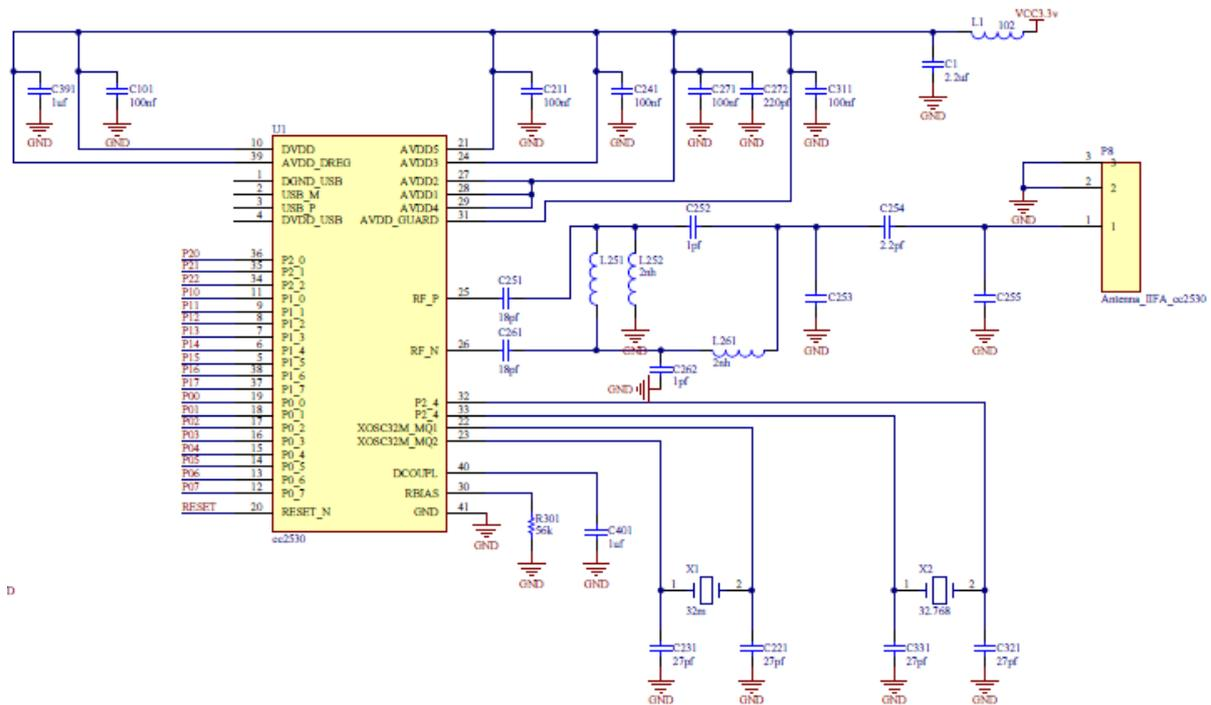
Fig. 6 (b). Main peripheral circuits of central node.
