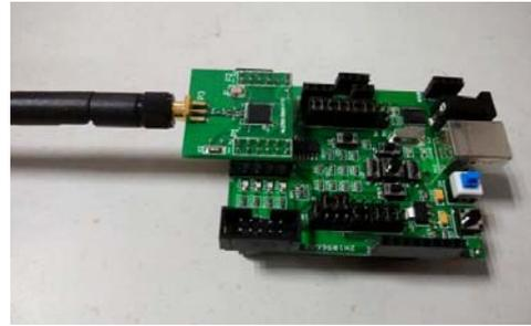
Fig. 6 (a). The manufactured sensor node picture.
