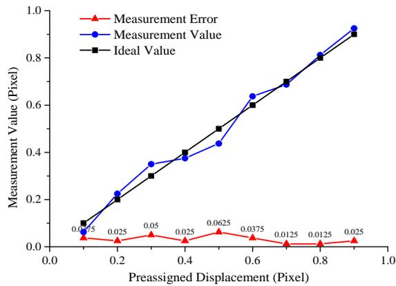
Fig. 6. The measurement results and error curve presented by the proposed algorithm.
