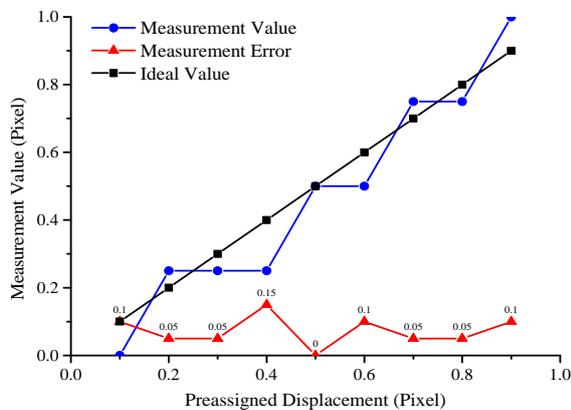
Fig. 7. The measurement results and error curve presented by the bicubic interpolation with the DSCM in spatial domain.
