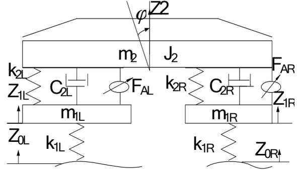
Fig. 1. Simplified single axle model of active suspension system.
