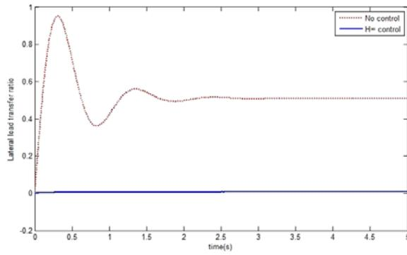
Fig. 6. Curves of rollover factor vs. time.
