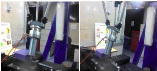
**Fig. 1.** 3-DOF parallel robotic machine tool developed in the R&A Lab in UOIT.
