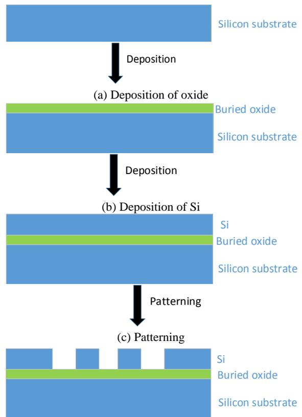
Fig. 6. Fabrication process.
