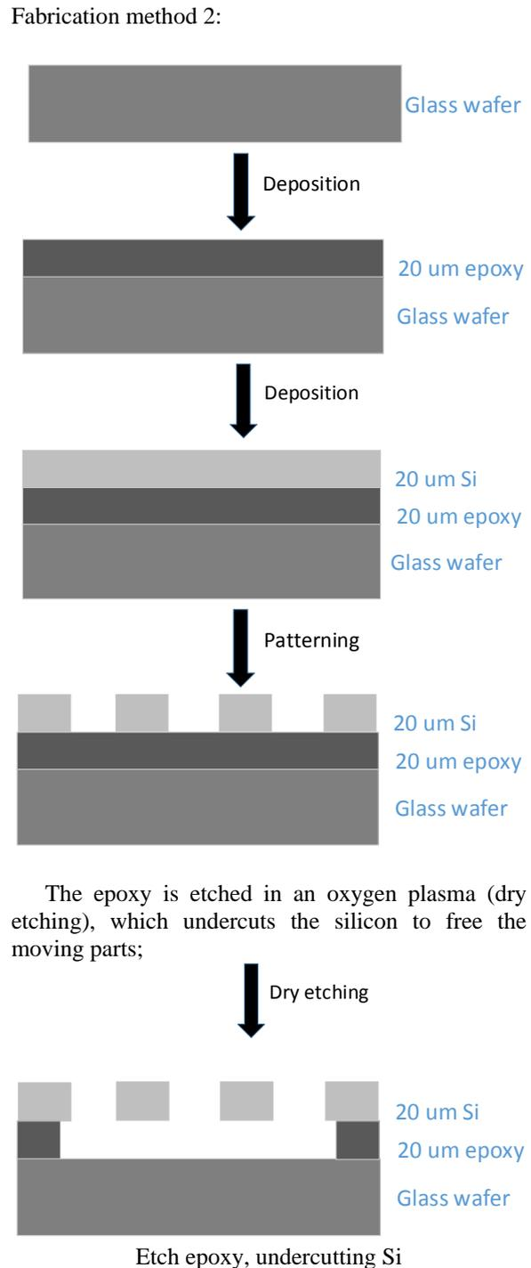
Fig. 7. Fabrication process.
