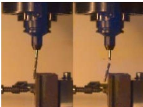
**Fig. 2.** Collision occurred during machining [10].
