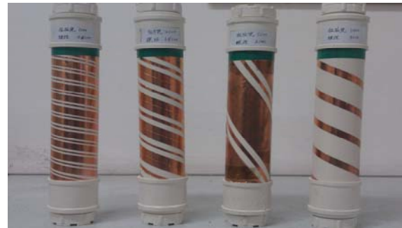
Fig. 2. Four sensor electrode structure.
