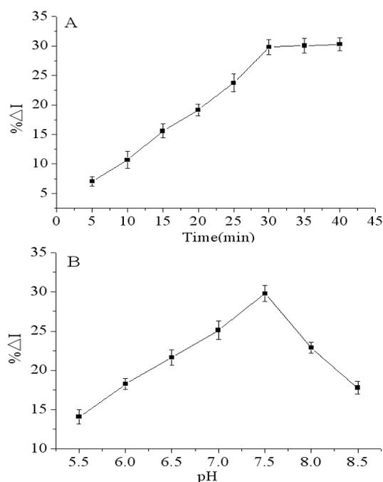
**Fig. 5.** Effect of incubation time (a) and pH of the detection solution (b) on the immunosensor.
