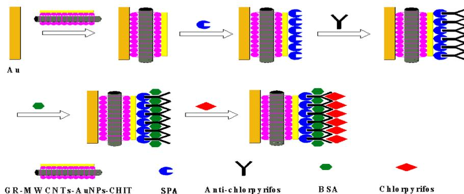
Fig. 1. Schematic illustration of the immunosensor fabrication process.
