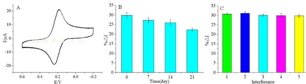
**Fig. 7.** (a) The stability analysis of immunosensor. (b) Decay of current response of the immunosensors with time. (c) The relative change in peak current (% $\Delta$ I) of proposed immunosensor to:
