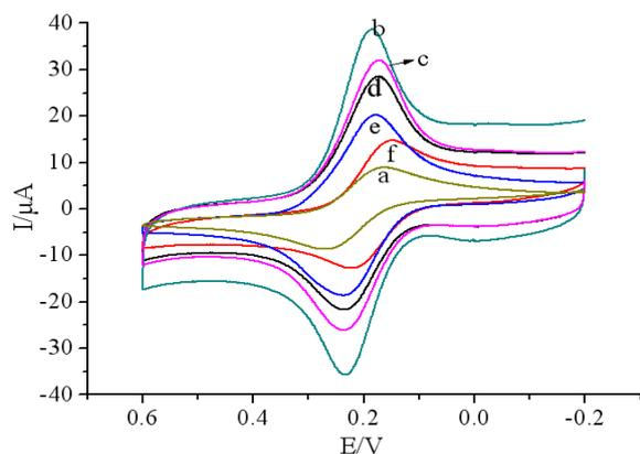
**Fig. 3.** Cyclic voltammograms: (a) bare Au; (b) GR-MWCNTs-AuNPs-CHIT/Au; (c) SPA/GR-MWCNTs-AuNPs-CHIT/Au; (d) anti-chlorpyrifos/SPA/GR-MWCNTs-AuNPs-CHIT/Au; (e) BSA/anti-chlorpyrifos/SPA/GR-MWCNTs-AuNPs-CHIT/Au; (f) chlorpyrifos/BSA/anti-chlorpyrifos/SPA/GR-MWCNTs-AuNPs-CHIT/Au recorded in pH 7.5 PBS containing 5.0 mM  $[\text{Fe}(\text{CN})_6]^{3-/4-}$  and 0.1 M KCl.
