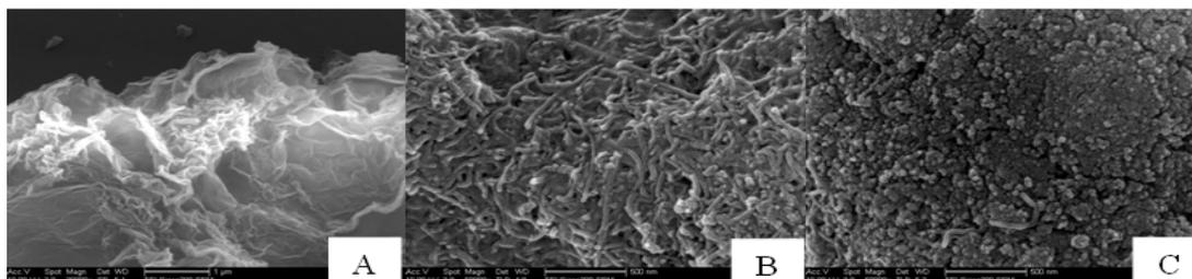
Fig. 2. SEM images of (A) GR, (B) GR-MWCNTs-CHIT and (C) GR-MWCNTs-AuNPs-CHIT.
