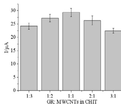
**Fig. 4.** Effect of the concentrations of GR-CHIT and MWCNTs-CHIT on the immunosensor.
