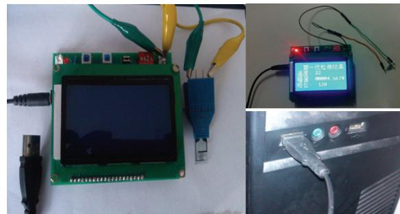
Fig. 8. Biosensor connected with rapid detection instrument.
