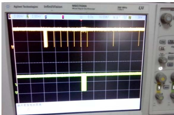
Fig. 10. Waveform of FPGA verification about Inventory.
