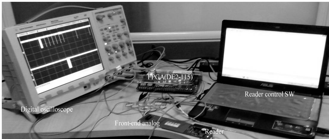
Fig. 9. FPGA validation test platform.
