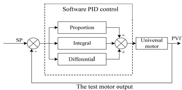
Fig. 2. Closed-loop PID structure diagram.
