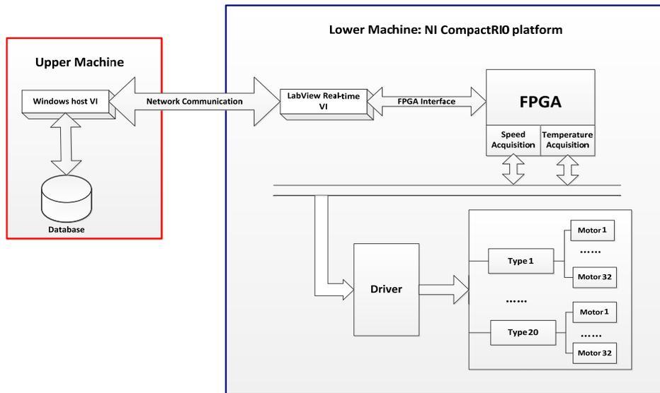
Fig. 3. Universal motor performance test block diagram.
