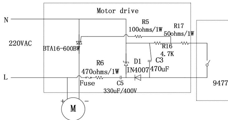
Fig. 4. Motor speed control principle diagram.
