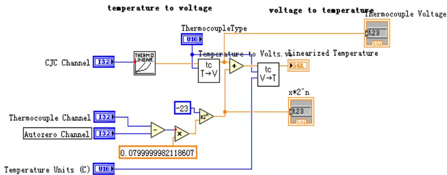
Fig. 9. Temperature conversion module block diagram.
