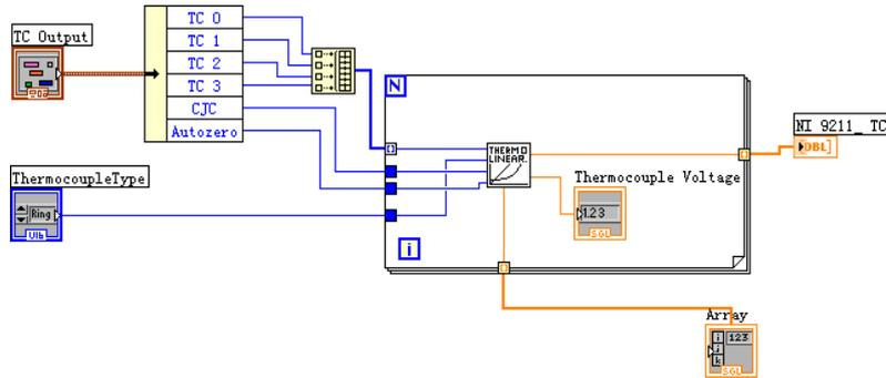
Fig. 8. Temperature measurement module block diagram.
