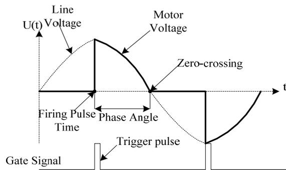
Fig. 1. Diagram of phase angle control.
