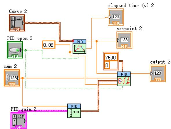
Fig. 6. PID control module block diagram.
