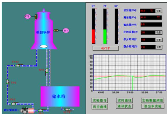
Fig. 7. PID control based on immune particle swarm subject to external interference.
