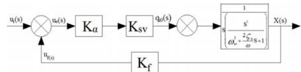
Fig. 2. System transfer function block diagram.
