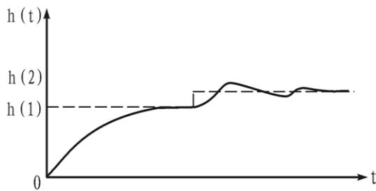
Fig. 8. The boiler liner water step response curves.
