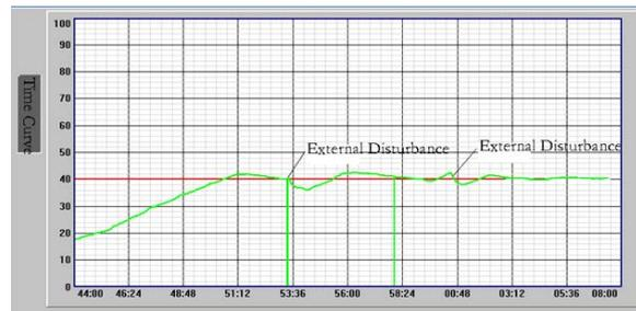
Fig. 9. Servo press hydraulic system control process curve.
