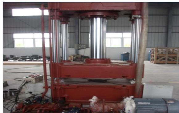
Fig. 10. The boarded of NC servo press hydraulic system.
