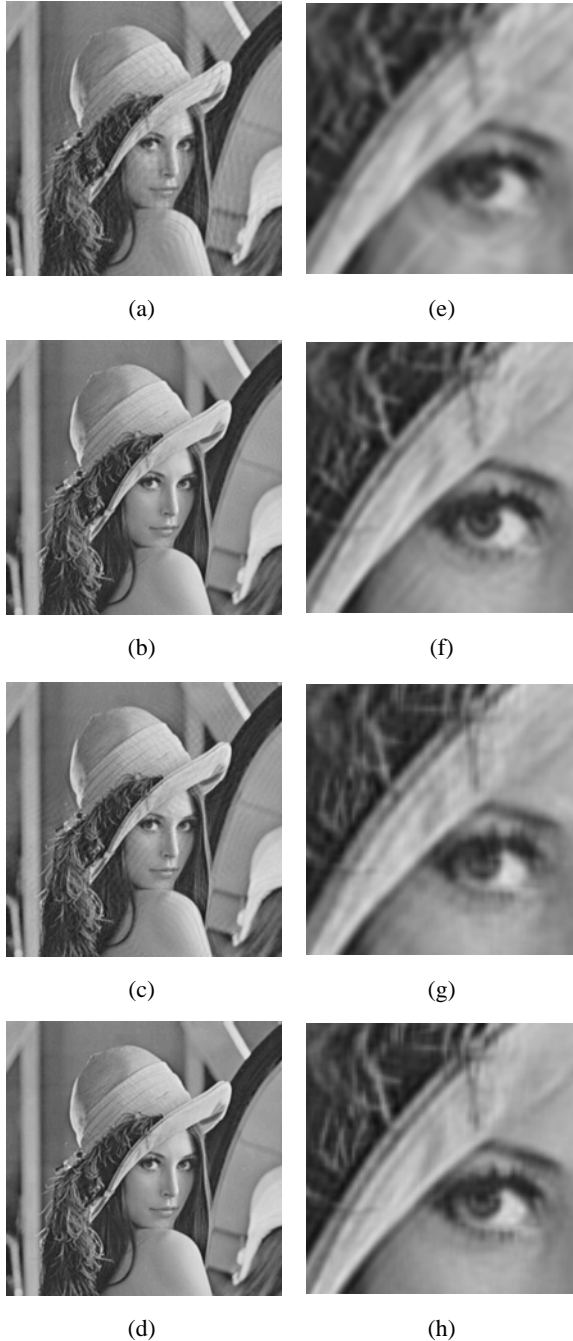
Fig. 6. Comparison of deblurring algorithms with LENA: (a) deblurred LENA image by classical Richardson-Lucy method; (b) deblurred LENA image by proposed disk multiple aperture method; (c) deblurred LENA image by Levin's method; (d) deblurred LENA image by proposed coded multiple aperture method; (e-h) details of restored images with above method.
