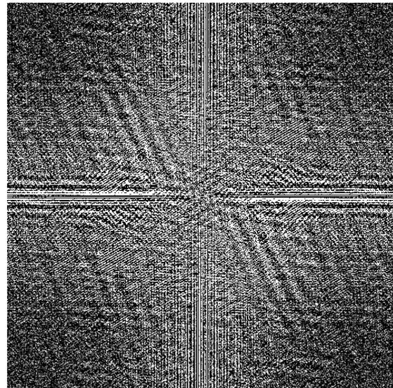
Fig. 3. Frequency spectrum of froth image with DC component shifted to center.
