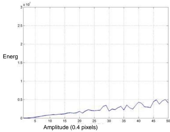
Fig. 11. Spectrum energy statistics of froth image with large bubbles.
