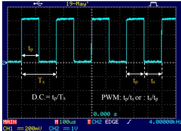
**Fig. 1.** Difference between duty-cycle and PWM informative parameters.
