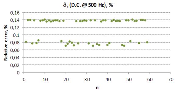
**Fig. 5.** Relative errors for duty-cycle measurements of 500 Hz input signal.
