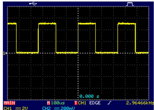
**Fig. 8.** Temperature sensor SMT16030's output at  $24.4\text{ }^{\circ}\text{C}$ : 44.21 % duty-cycle, 2 964.66 Hz at  $V_{cc}=4.97\text{ V}$ .
