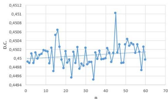
**Fig. 9.** Duty-cycle values at 60 measurements for the temperature  $+24.4^{\circ}\text{C}$ .
