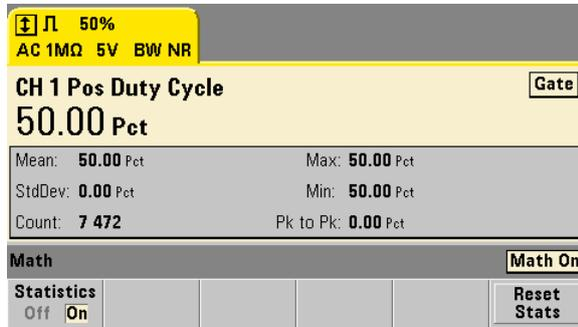
**Fig. 2.** Conventional true value for duty-cycle measurement (D.C. = 50 % at 500 Hz).
