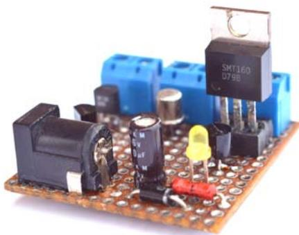
**Fig. 6.** Temperature sensors SMT16030 from *Smartec* (The Netherlands) on investigation board.
