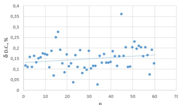
**Fig. 10.** The relative error of duty-cycle measurement.
