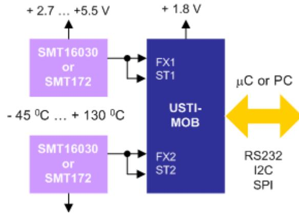
**Fig. 7.** Low power consumption temperature sensor systems.
