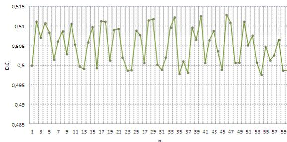
**Fig. 3.** Results of measurements for duty-cycle of 100 kHz input signal.
