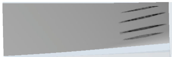
Fig. 18. Contact trajectory of the same tooth surface with positive installation error.
