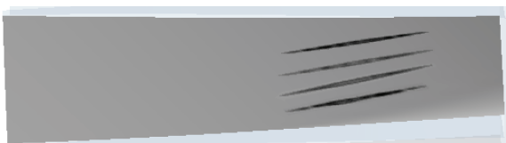
Fig. 20. Contact trajectory of the same tooth surface with negative installation error.
