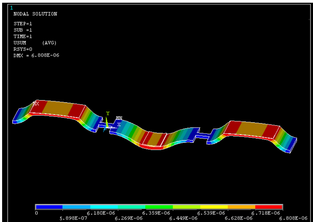
Fig. 7. Deflection of serial actuators at applied 105 V.
