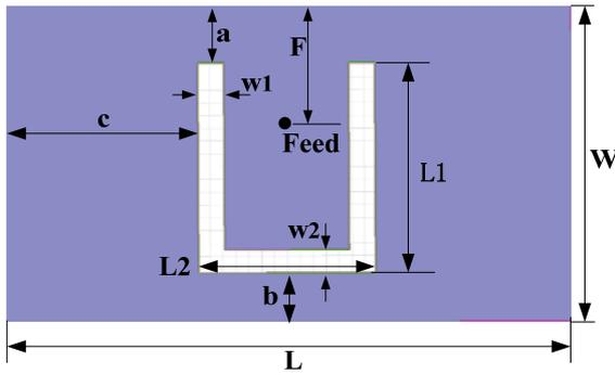
Fig. 1. The schematic diagram of slotted patch antenna.
