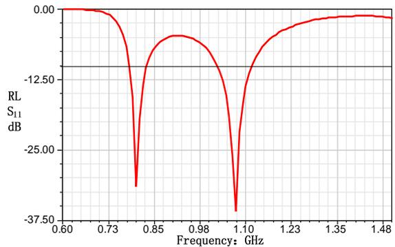
Fig. 2. The relationship between the antenna return loss and frequency.
