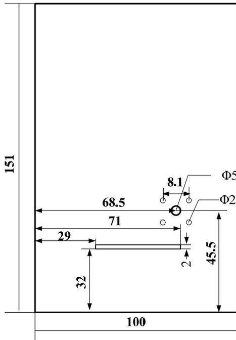
Fig. 7. The schematic diagram of antenna ground plate.
