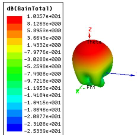
Fig. 3. The 3D gain pattern of the antenna.
