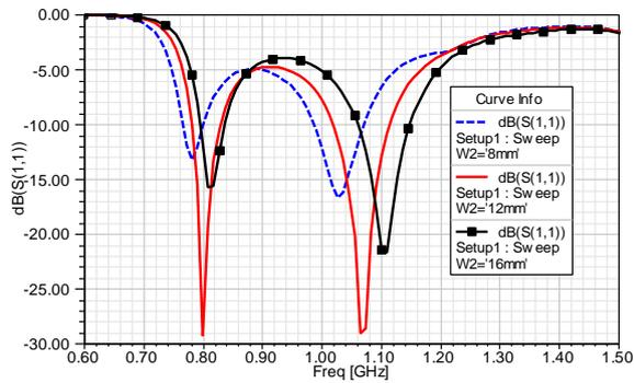
Fig. 4. The relationship between the antenna return loss and frequency with different  $W_2$ .
