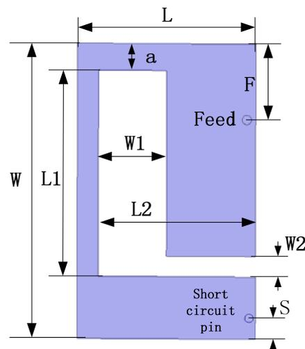
Fig. 6. The schematic diagram of antenna patch.
