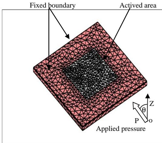
Fig. 1. Model of elastomeric membrane and boundary conditions
