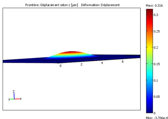
Fig. 6. Deformation of PMMA membrane induced by applied pressure with  $\theta = 0^\circ$ .
