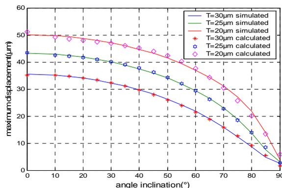
Fig. 10. Maximum of Displacement on Surface of PMMA to Different Values of Inclination Angle.
