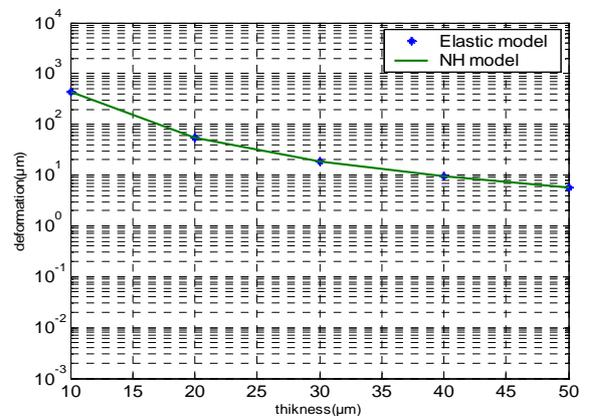
Fig. 5. Maximum of vertical displacement on surface of PDMS membrane at different thickness.
