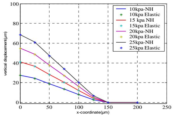
Fig. 3. Vertical displacement on surface of PDMS membrane at different pressure: comparison between N- Hookeen and Linear model.
