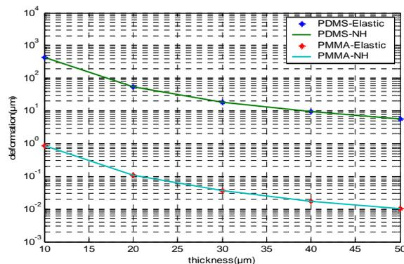
Fig. 9. Maximum of Vertical Displacement on Surface of PDMS and PMMA Membrane at Different Thickness.
