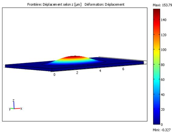
Fig. 2. Deformation of PDMS membrane induced by applied pressure with  $\theta=0^\circ$ .
