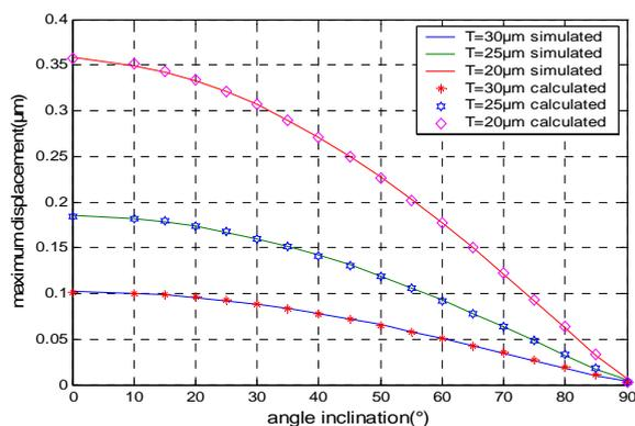
**Fig. 11.** Maximum of Displacement on Surface of PMMA to Different Values of Inclination Angle.
