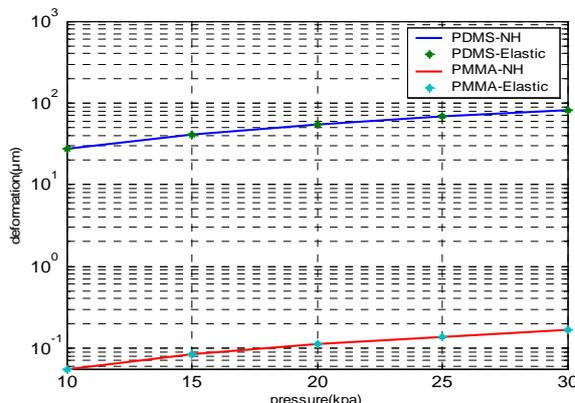
Fig. 8. Maximum of Vertical Displacement on Surface of PDMS and PMMA Membrane at Different Pressure.
