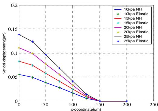
Fig. 7. Vertical Displacement on Surface of PMMA Membrane at Different Pressure: Comparison between N-Hookeen and Linear Model.
