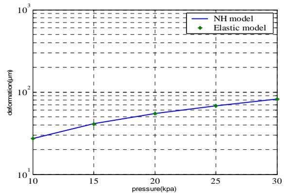
Fig. 4. Maximum of vertical displacement on surface of PDMS membrane at different pressure.
