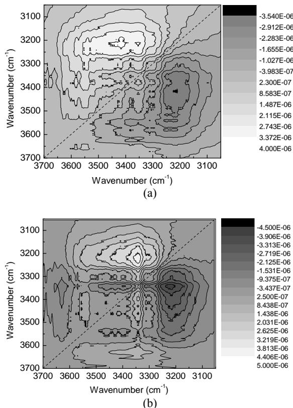
Fig. 5. Asynchronous correlation spectrum of vegetable and mineral oil-impregnated paper.
