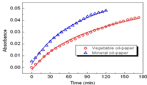
Fig. 6. Fitting curves of absorbed water in oil-paper insulation.
