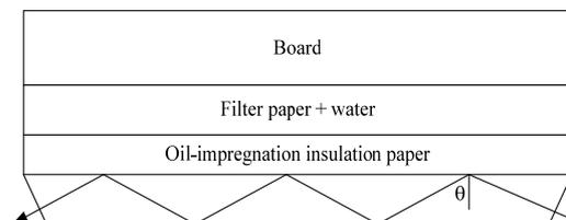
Fig. 1. Schematic description of the ATR-FTIR experimental arrangement.
