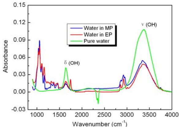
**Fig. 2.** ATR-FTIR spectra of absorbed water in oil-impregnated insulation paper.
