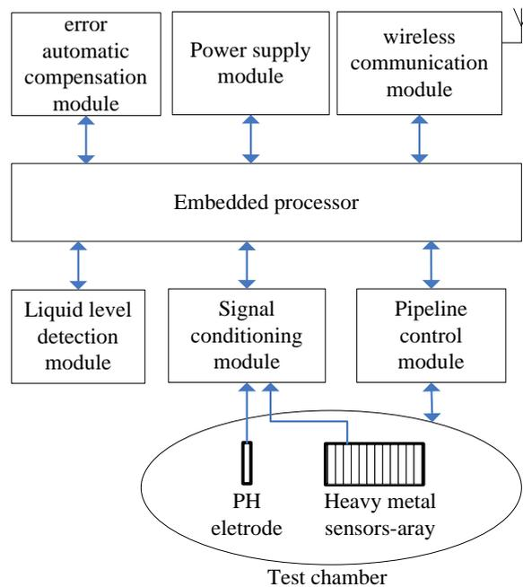
Fig. 2. Hardware block diagram of monitoring terminal.
