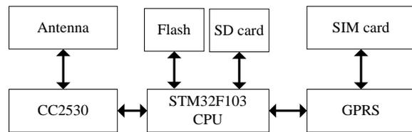
Fig. 3. Hardware block diagram of gateway.
