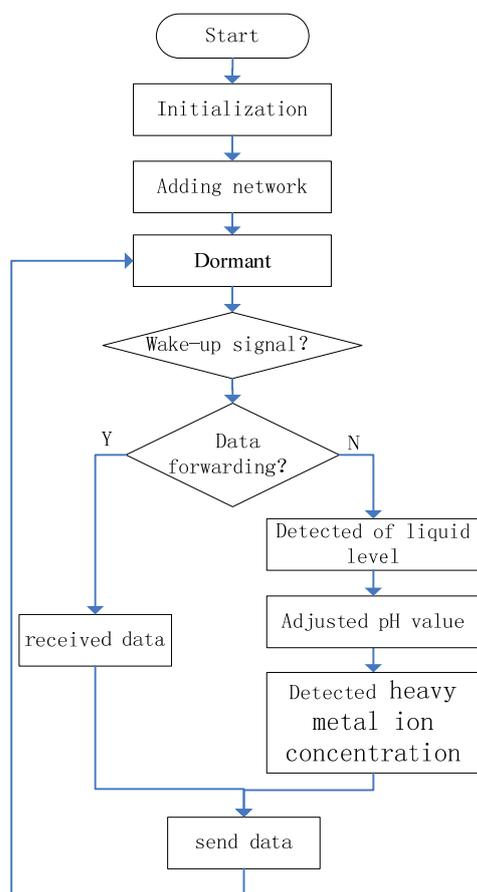
Fig. 5. Monitoring terminal program flow chart.
