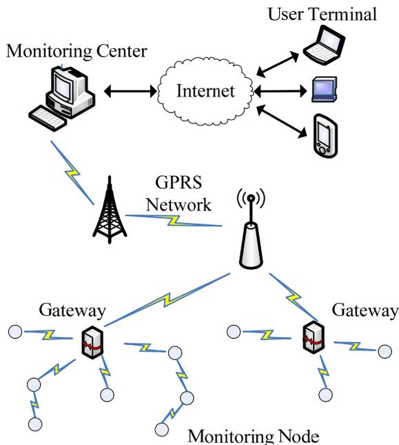
Fig. 1. Structural diagram of the system.
