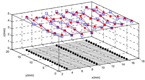
**Fig. 8.** Decoupling results based on the RBFNN with WGN. The blue square represents the initial deformation for the electrodes on the upper layer of the sensor, and the red circle represents the decoupling deformation correspondingly.
