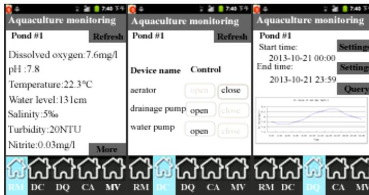
Fig. 5. Main control interface of aquaculture monitoring on Android platform.
