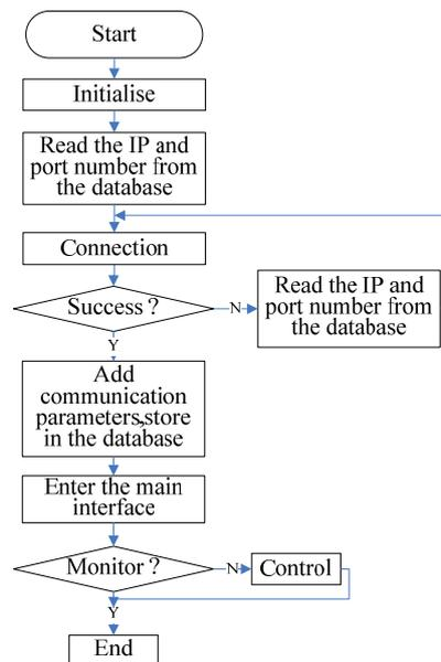
Fig. 4. Main control flow chart of aquaculture monitoring on Android platform.
