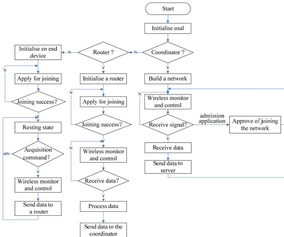
Fig. 2. ZigBee network flow chart of main program.
