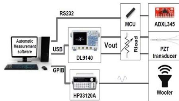
Fig. 4. Measurement bench for the characterization of the piezoelectric transducer.
