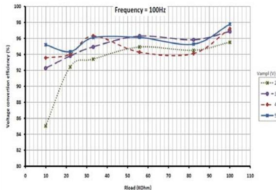
Fig. 12. Voltage conversion efficiency of the designed active rectifier for an input signal of 100 Hz frequency and varied amplitudes.
