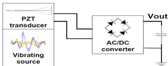
Fig. 1. Block diagram of a simple vibration-based piezoelectric energy harvesting system.
