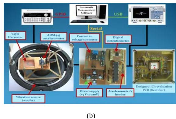
Fig. 2. Measurement bench for the characterization of the energy harvesting system: a) Block diagram and b) Setup.
