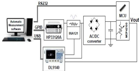
Fig. 5. Measurement Bench for the characterization of the designed active rectifier.
