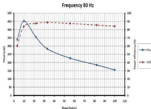
Fig. 15. Output power and power efficiency of the EH system for different resistive loads.
