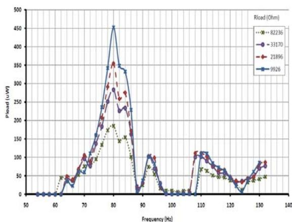
Fig. 14. Harvested power for varied frequencies and loads.
