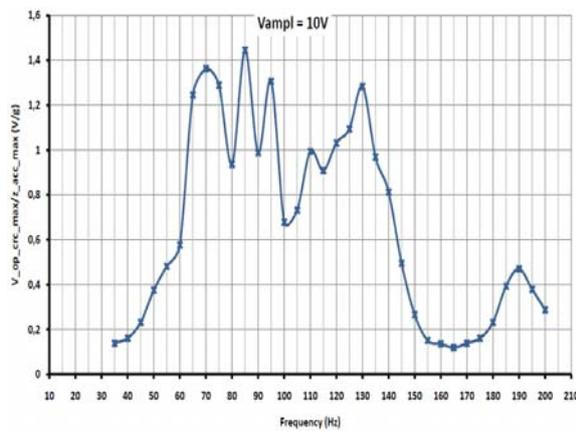
Fig. 9. Normalized open circuit voltage of the transducer for varied frequencies of the excitation signal (V<sub>ampl</sub>=10 V).
