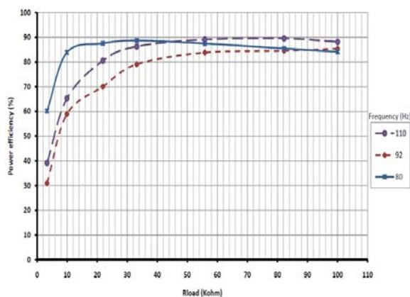
Fig. 13. Power efficiency of the EH system for varied resistive loads and selected frequencies.
