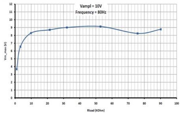
Fig. 10. Maximum output voltage of the harvester for varied resistive loads (excitation signal: 10 V, 80 Hz).
