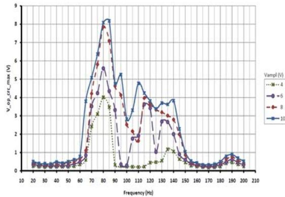
Fig. 8. Maximum open circuit voltage of the transducer for varied amplitudes and frequencies of the excitation signal.
