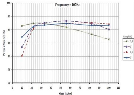
Fig. 11. Power efficiency of the designed active rectifier for an input signal of 100 Hz frequency and varied amplitudes.
