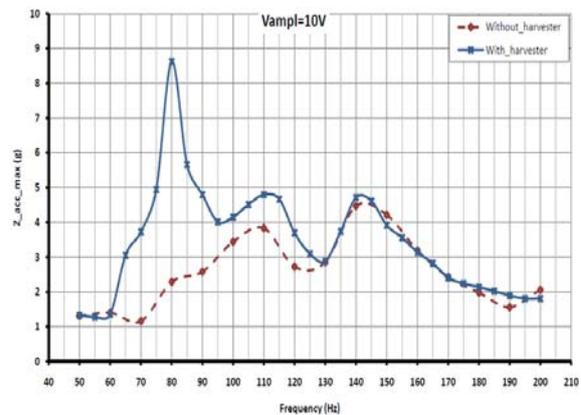
Fig. 7. Z-axis vibration spectrum of the source with and without the harvester, for the maximum available amplitude (10V) of the excitation signal.
