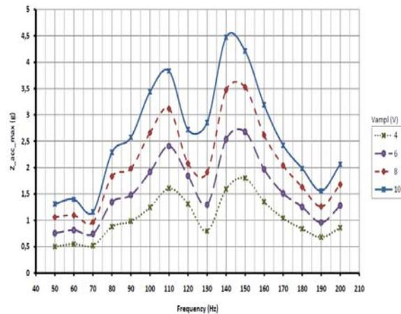
Fig. 6. Maximum detected z-axis acceleration magnitude of the vibration source for different amplitudes and frequencies of the excitation signal.
