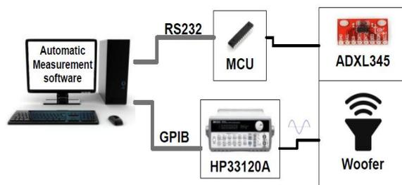
Fig. 3. Measurement bench for the characterization of the vibrating source.
